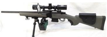
**VARIANTS:** Various rifles of different brands and models may be ergonomically improved with the fitting of an adjustable cheek piece. Consideration for proportional need of an adjustable cheek piece is the sighting system used, and the sight height in relation to the eye height of the firer after forming a solid cheek weld.
